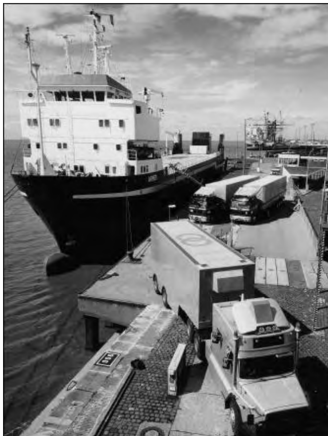
Figure 3. The “Arneb”, a Ro-Ro vessel licensed for INF2 and security category I shipments.
