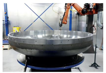
Figure 2. Diode laser cladding processing of a pressure vessel lower dome (NAMRC)
