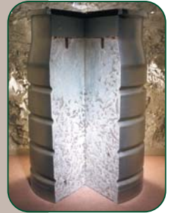
ILW packaged and conditioned in a 500l drum
